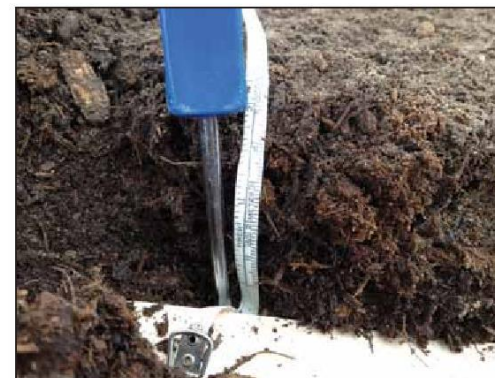
Section 83.3.5 states, "Mulch, soil, and other materials should be removed as needed to allow for inspection." After fresh mulch was removed, a 2" layer of compacted mulch remained above the soil. No root growth was found in this shredded hardwood, which looked and smelled as sterile as peat.
